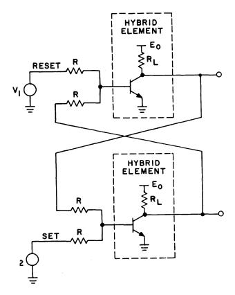
Figure 7—Set-reset flip-flop
