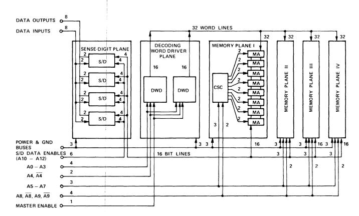
Figure 13-8192 bit memory stack-electrical organization
