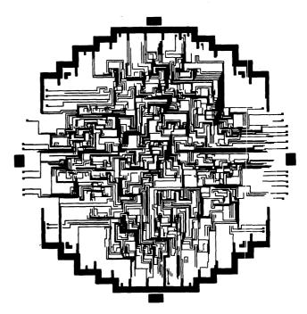
Figure 17—5-bit modular multiplier standard interconnect mask
