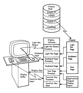
Figure 10-Display control interface
