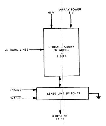
Figure 2—Block diagram MOS storage array
