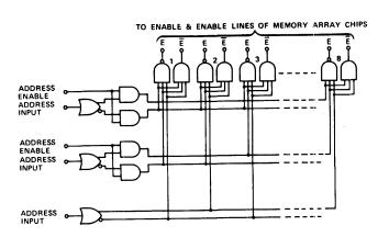
Figure 6—Chip select circuit logic
