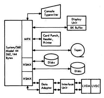
Figure 2—Flight software development laboratory—Block diagram
