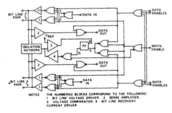
Figure 11—Sense amplifier/digit driver chip logic
