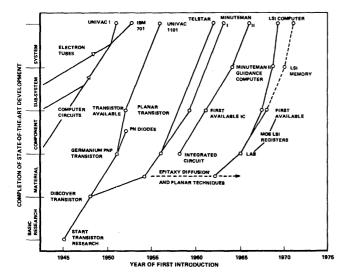
Figure 6—Tracing the development of new components into systems
