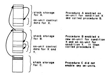
Figure 7—Stack storage and the signal mechanism A signal for condition X causes the signal mechanism to search tack through the stack until it finds the first enabled on-unit for condition X.
