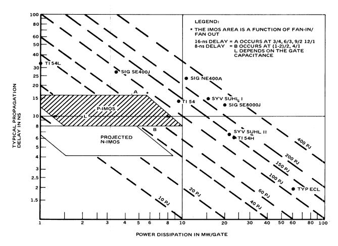
Figure 7-Speed-power products of some bioplar and MOS circuits
