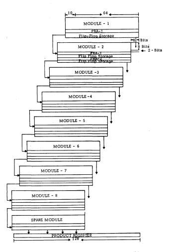
Figure 8—Example of an assembled  $64 \times 64$ -bit multiplication unit using the pipelining scheme
