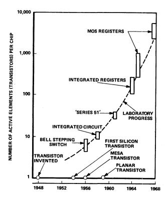
Figure 1—Complexity of integrated circuits versus year of laboratory accomplishment
