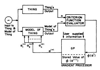
Figure 1—Application of the gradient processor element to parameter identification
