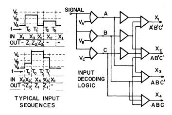
Figure 6—Shock measurement system — Front end
