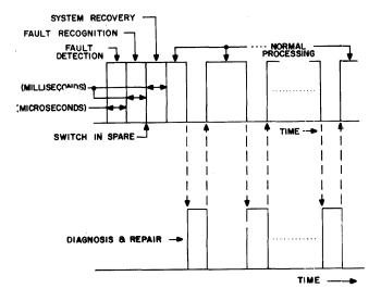
Figure 2—Fault recovery sequence (with spare)
