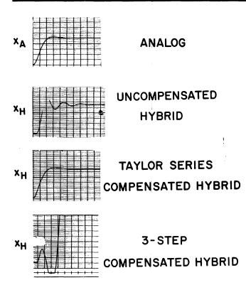
Figure 1—Strip chart records of x(t) for  $\omega = 0.412$ ,  $\zeta = -0.2425$ ,  $\zeta_T = 0.7$ ,  $\omega_T = 15$ . The sample interval T = 25 ms.
