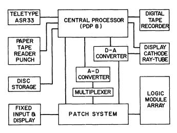
Figure 1—DADEC system — Block diagram
