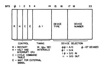
Figure 3—Hybrid processor commands
