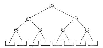
Figure 10—An alternate interconnecting scheme for the 8-modules of the 64 × 64 multiplication unit
