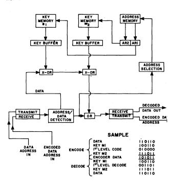
Figure 1—Digital substitution logic
