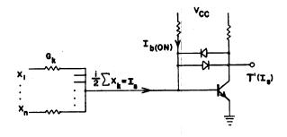
Figure 2—Threshold gate with Schottky diode feedback
