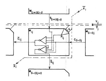
Figure 6-Functional multiplier cell
