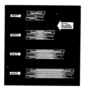
Figure 11--Four relocation patterns for SN5480's
