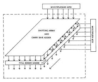
Figure 1—The integral parts of the asynchronous multiplication array
