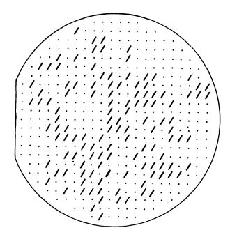
Figure 2—Wafer after test—Slashes show good circuit positions
