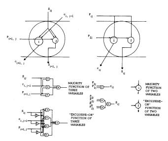
Figure 3a, b—Cell "S", Cell "C"
