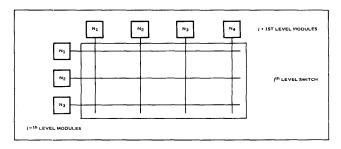
Figure 3—Module-switch-module relationships
