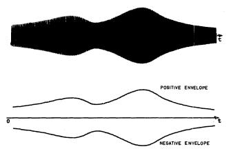
Figure 3—Typical data signal and the computer generated envelopes
