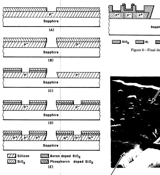
Figure 5—Low temperature CMOS Process
