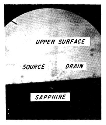
Figure 4—Photomicrograph of diffusion failure in SOS
