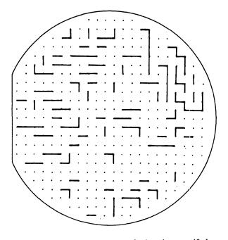
Figure 8—Mask pattern for the pad relocations specified in Figure 5
