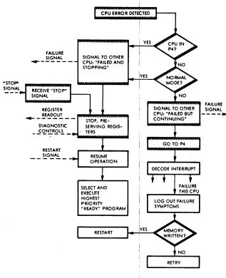
Figure 6--Central processor error: Failed CPU
