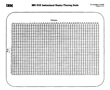
Figure 2—This shows the organization of the screen into 32 rows and 40 columns forming 1280 addressable units. The standard alphameric characters occupy two of these boxes, i.e., two rows by one column
