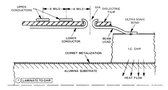
Figure 15-Interconnect cross-section
