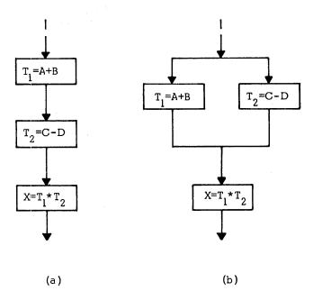
Figure 3—Illustration of parallelism within a compound task
