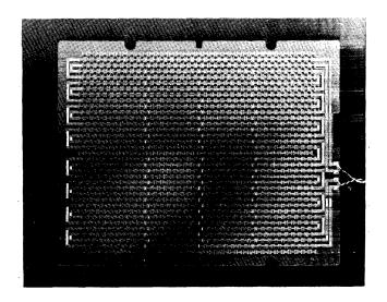
Figure 7—The mated film core array
