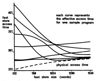
Figure 2—The physical assess time of a fast store (broken line) and the effective access times (continuous lines) for sample programs. Access time is a percentage of main store access time, storage size is in words, and line size is 4 words
