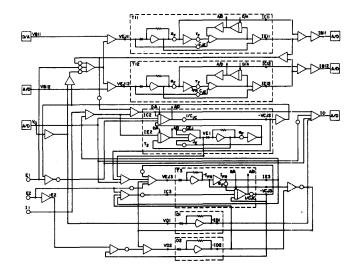
Figure 13—Analog computer simulation of a NOR gate
