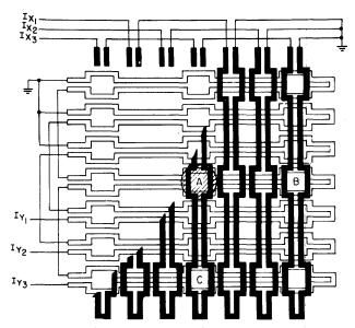
Figure 9—Thin film conductor pattern for two dimensional propagation of cylindrical domains. Conductor dimensions identical with that of Figure 6.
