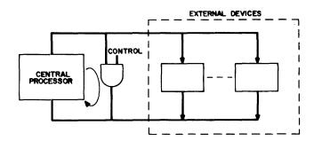
Figure 5b—Processor interface with external system (maintenance mode)
