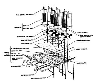
Figure 12—The substack
