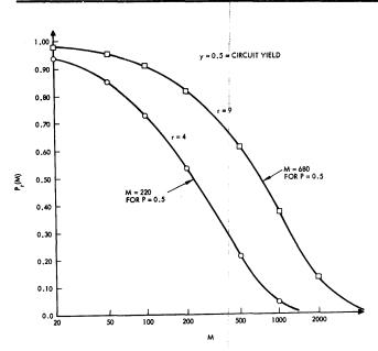
Figure 19—The probabilty  $P_r(M)$  of successfully fulfilling a master pattern of M circuits by relocating from one of up to r nearby circuits. Each circuit is a tested unit which may have many gates of logic complexity
