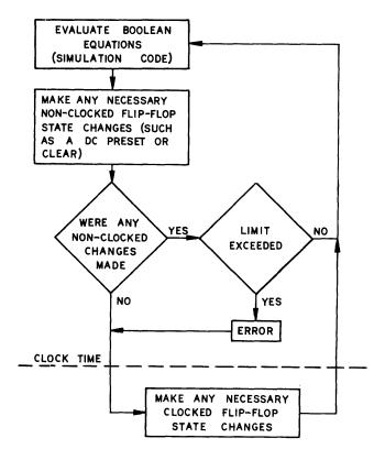
Figure 4—Simulator controller
