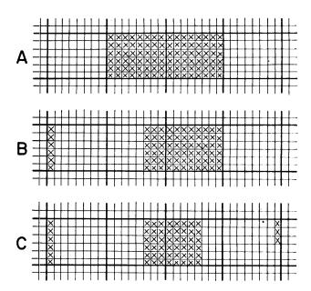
Figure 7—This shows the problem of erasure with multiple display inserts on the same row. The insertion of the single dot column in (B) causes erasure of 5 dot columns from the original pattern in (A). Insertion of the 1/2 dot column in (C) causes erasure of 3 dot column from the original pattern
