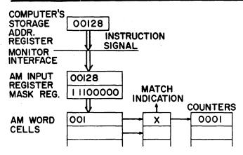
Figure 1—Assignment of counter to initial execution area
