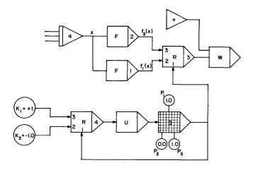
Figure 9—Storage element used to modify structure of simulation from one solution to next
