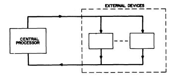
Figure 5a—Processor interface with external system (operational mode)
