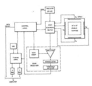
Figure 4—Position encoder block schematic
