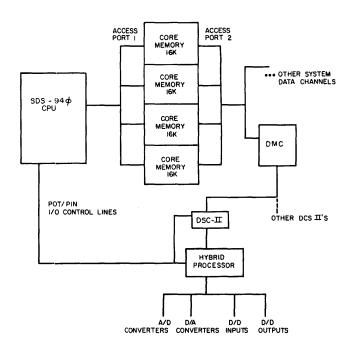
Figure 5-Connection of hybrid processor to SDS-940
