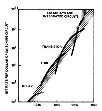
Figure 5—Switching rate per dollar for computer logic elements
