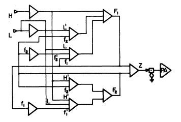
Figure 3—Pulse-height detector — Logic diagram
