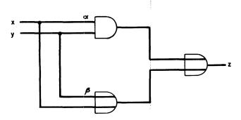
Figure 6—Example of a redundant circuit
