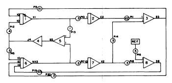
Figure 2—Simulation of an automobile suspension system
