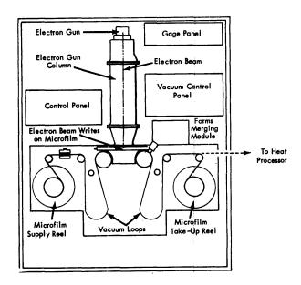
Figure 6-Electron beam recording on microfilm
