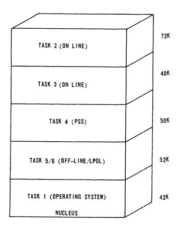
Figure 11—Initial task core allocations
