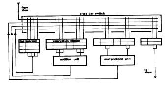
Figure 5—Typical floating point unit for use with Tomasulo's algorithm
