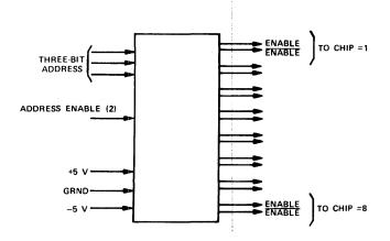
Figure 5—Chip select circuit
