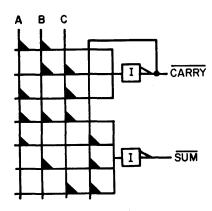
Figure 8—SLT full adder position
