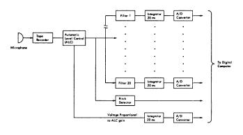
Figure 2—Functions of analyzing hardware
