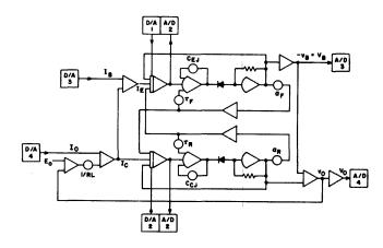
Figure 10-Analog simulation of a NOR gate
