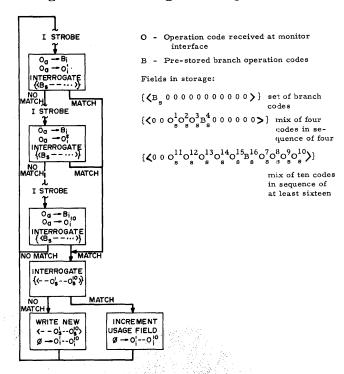
Successive operation codes are placed in successive O fields across the I/E register by means of a string of macroinstructions differing only in the routing
