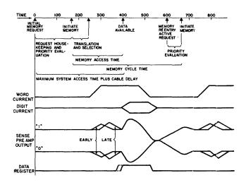
Figure 17—Timing for a typical memory cycle
