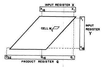
Figure 5-16 × 16 bit functional multiplier
