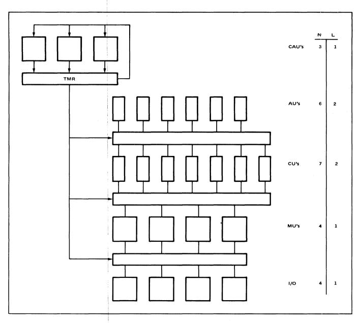
Figure 5-Multi-module modular computer
