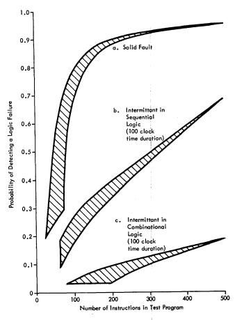
Figure 5—Efficiency of test program vs. program size
