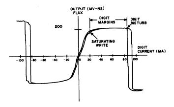
Figure 5-Output flux vs. digit current
