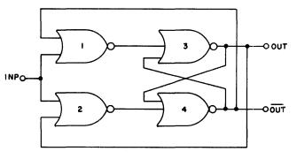
Figure 11-Trigger flip-flop
