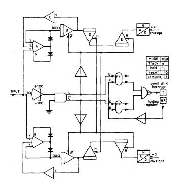
Figure 4—The envelope detection circuit
