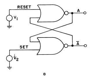
Figure 6a-Set-reset flip-flop
