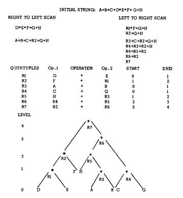
Figure 12—Parallel computation of A+B+C+D\*E\*F+G+H using Squire's algorithm
