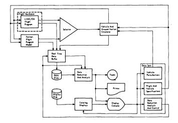
Figure 7—Application software functional flow— Real-time phase
