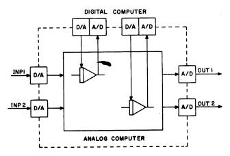
Figure 2—The hybrid element
