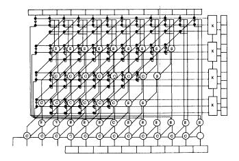
Figure 6—The binary multiplying cellular array
