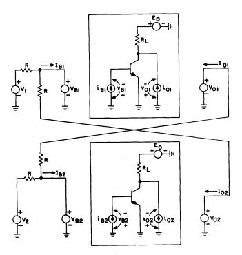
Figure 8—Set-reset flip-flop
