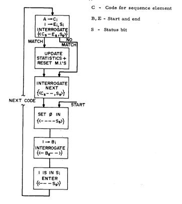
Initially, and at the end of each cycle, the status bits are set to one for all first elements.
