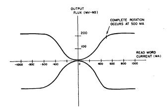
Figure 4—Output flux vs. read word current
