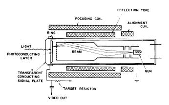
Figure 2-Schematic cross-section of the vidicon
