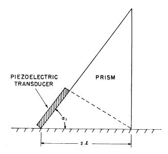
Figure 1—Surface wave radiator/sensor
