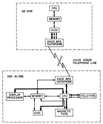
(THIN LINES REPRESENT DATA TRANSMISSION; HEAVY LINES REPRESENT TRANSMISSION OF STATUS INFORMATION AND INTERRUPTS)
