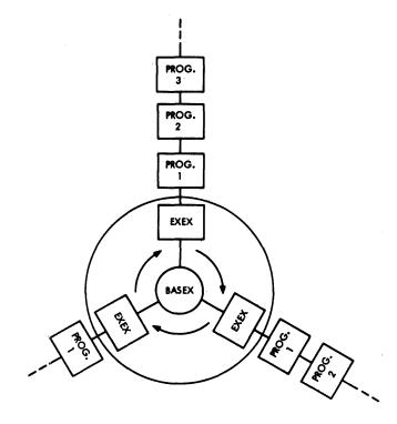
Figure 3—Simple commutation of users programs. This figure illustrates the relationship between user's programs' EXEX and BASEX. Each spoke represents a user's job, with his EXEX providing the interface between BASEX and the hardware resources. The maximum number of interactive job the IBM 360/50H configuration is ten.
