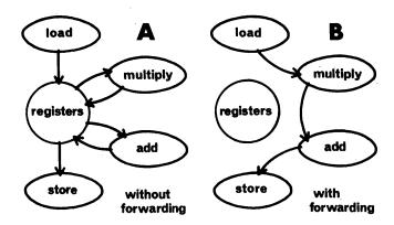
Figures 4a and 4b—The use of forwarding to speed arithmetic calculations
