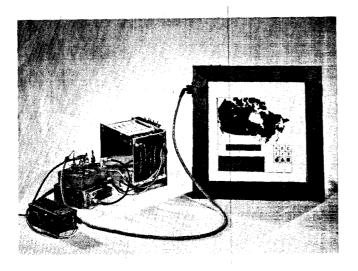
Figure 6—Touch sensitive position encoder
