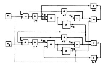
Figure 9—HYPAC block diagram for set-reset flip-flop
