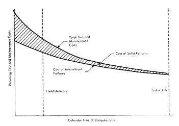
Figure 7—Cost of failures
