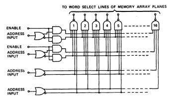
Figure 9—Decoding word driver chip logic
