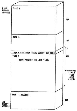
Figure 2—Showing memory configuration when low priority on line (LPOL) task is active
