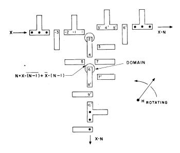
Figure 17—Cylindrical domain flip flop—The state of the flip flop is determined by the presence or absence of a trapped circulating domain at the sequencing pole positions; (idler) 4, 5, 6, 7. Each new domain entering the input channel x changes the state of the flip flop by becoming trapped in the idler if it is full
