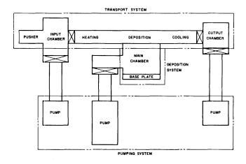
Figure 10—Continuous vacuum evaporator
