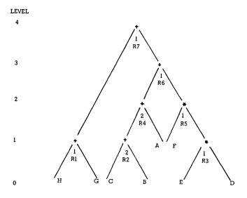
Figure 14—Binary tree for parallel computation of A+B+C+D\*E\*F+G+H
