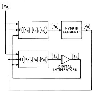
Figure 4—Principle of operation of HYPAC
