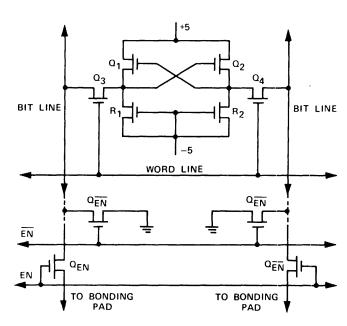
Figure 3—Storage cell circuit schematic
