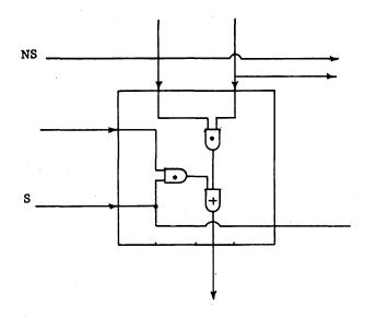
Figure 7b—Cell "R"—Reconfiguration cell
