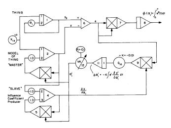
Figure 6—MOBSSL block diagram demonstrating use of VK block as iterative element in parameter search by discrete sensitivity difference equation technic
