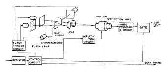
Figure 1-Schematic diagram of the character generator
