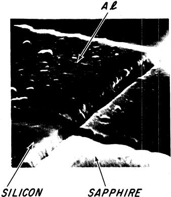
Figure 7—Aluminum metallization over oxidized silicon edge
