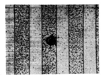
a-2. Enlargement showing self-healed pinhole
