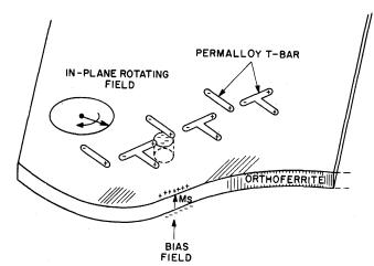
Figure 14—Isometric view of permalloy T-BAR pattern in contact with surface of orthoferrite platelet. Rotating in-plane field generates poles which cause the domain to move
