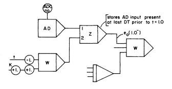
Figure 12-AD block used to modify a parameter at the beginning of a run
