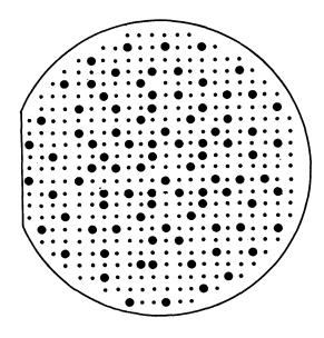
Figure 3—A master pattern of good circuits—All wafers will be matched to this pattern by the Pad Relocation technique
