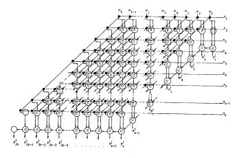
Figure 2—The "single-bit" asynchronous multiplication cellular array
