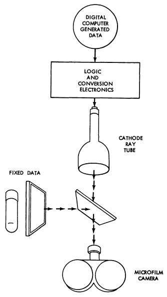
Figure 5-CRT microfilm recording
