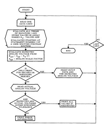
Figure 4-Static check control
