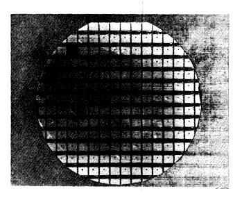
Figure 2—Map of wafer of 256-bit shift registers
