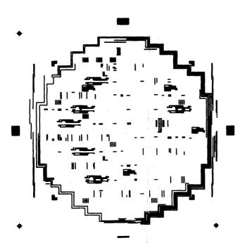
Figure 16—Pad relocation mask with standard crossunders
