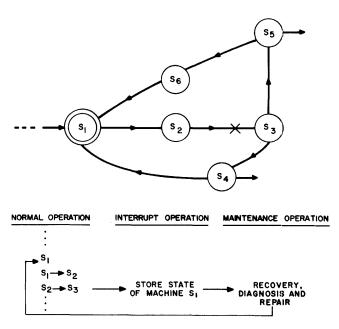
Figure 4—The use of interrupt and rollback mechanisms
