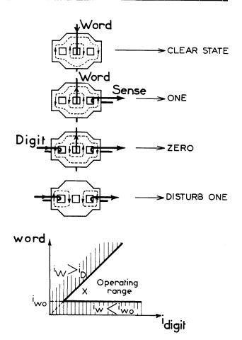
Figure 2—Operation of the three hole element
