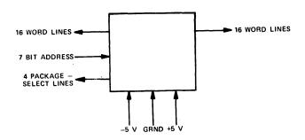
Figure 10-Decoding word driver package
