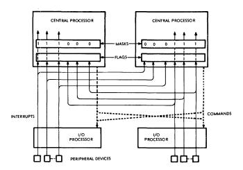
Figure 4—Input-output control block diagram
