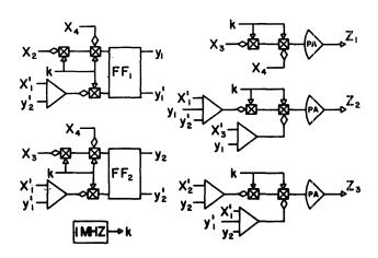
Figure 8—Shock measurement system — Logic diagram
