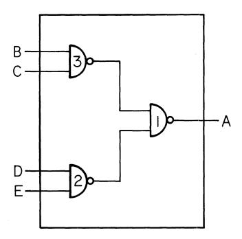
Figure 8—Logic module as defined for partitioning purposes
