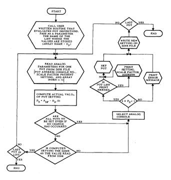
Figure 3—Potentiometer setting control
