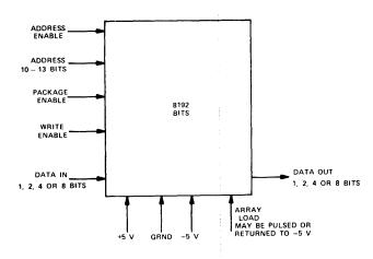
Figure 1-Block diagram 8192 bit module
