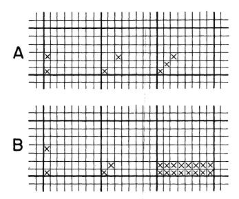
Figure 8—(A) shows three dot patterns which permit light pen detection; (B) shows three dot patterns which would not be detected by the light pen
