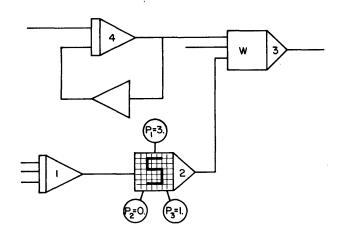
Figure 8—Use of storage element to store and transfer integrator output between simulations during iterative operation
