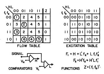
Figure 2—Pulse-height detector — Description
