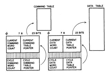
Figure 4—Command and data table structure
