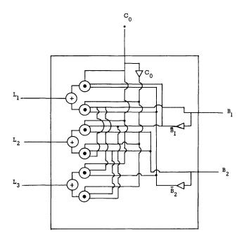
Figure 5b—Cell-K of the input control circuit
