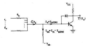
Figure 1—Modified RTL gate with tunnel diode feedback
