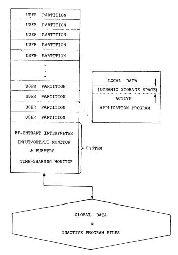
Figure 1—A schematic diagram of the core memory allocation of the MUMPS system and user partitions. A single partition is expanded to show its internal structure. The use of secondary storage (disk) for global data and inactive programs is represented.
