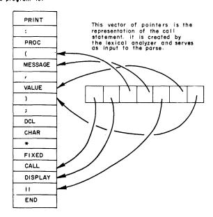
Figure 2—The output of the lexical analyzer.
