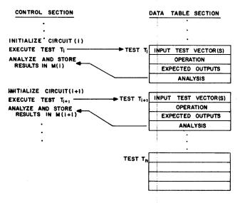
Figure 7—Layout of a diagnostic program structure
