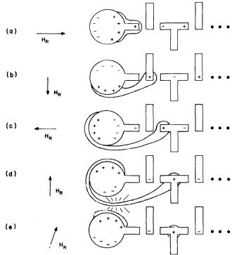
Figure 16—Domain generation—A permanent domain associated with the rotating + pole configuration of the generator disk is forced to stretch when one end becomes trapped in the T-BAR propagate channel. When the in-plane rotating field  $H_R$  is directed upward, the - poles near the stretched portion of the domain cause it to sever into two, leaving a newly formed domain in the propagate channel
