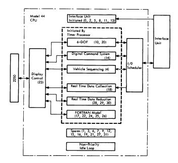
Figure 8—Functional groupings of priority interrupt line assignments (0-31) in real-time phase
