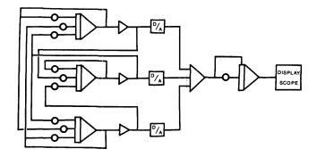
Figure 5-Linear PDE problem analog diagram
