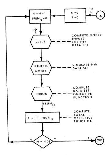
Figure 7—Simplified objective function flow diagram
