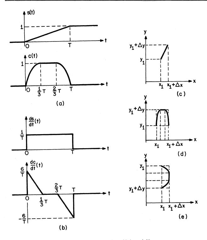
Figure 6—Waveforms for straight/cusp primitives
