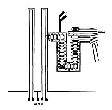
Figure 10—Photograph of the conductor pattern of a undirectional shift register utilizing a biphase propagating source. The circuit contains a controlled replicate input and an output circuit which detects a change in flux. Circuit is capable of propagating domains having a nominal diameter of 4 mils
