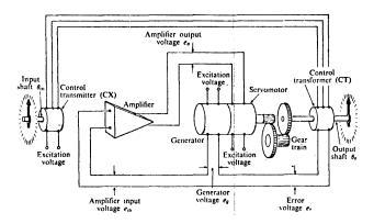
Figure 4—Schematic diagram of motor-generator instrument servomechanism
