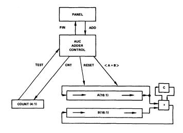
Figure 3—Serial adder
