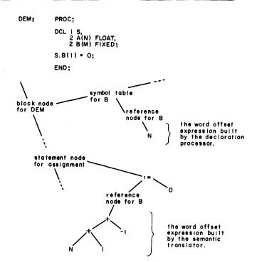
Figure 5—A simplified diagram showing the effects of subscripting
