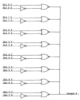
Figure 4—Hardware to test if X is a subset of Y  $Z = (\widetilde{Y}_0 \wedge X_0) \vee (\widetilde{Y}_1 \wedge X_1) \vee \ldots \vee (\widetilde{Y}_7 \wedge X_7)$
