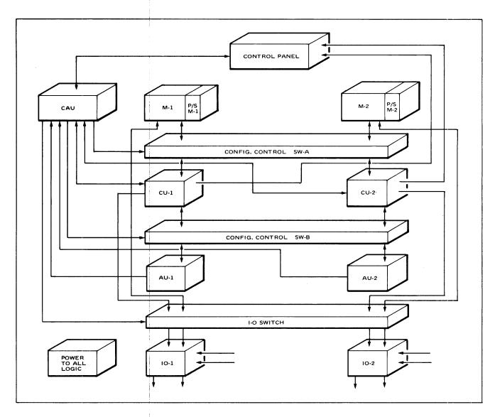
Figure 1-Modular computer breadboard
