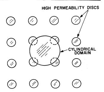
Figure 5—Interaction between a matrix of high permeability disks and a cylindrical domain
