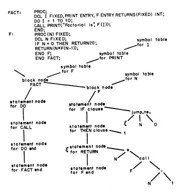
Figure 1—The internal representation of a program. The example is greatly simplified. Only the statements of procedure F are shown in detail.
