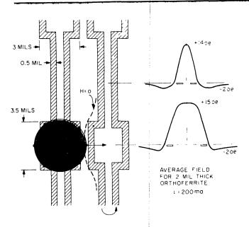
Figure 6—Conductor circuit used to propagate cylindrical domains and the resulting field profiles for 200 mA applied current
