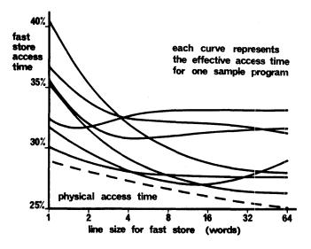
Figure 3—The physical access time of a fast store (broken line) and the effective access times (continuouslines) for several sample programs. Access time is a percentage or main store access time line size is in words, and store size is 1024 words
