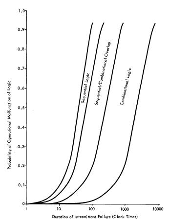
Figure 3-Sensitivity of arithmetic logic
