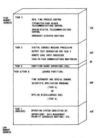
Figure 1—Initial memory configuration with task functional descriptions and relative locations shown
