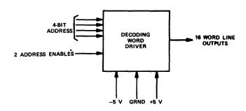
Figure 8—Decoding word driver chip
