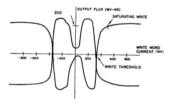
Figure 6—Output flux vs. write word current
