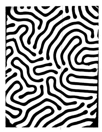
Figure 1—Strip domains, 1.5 mils in width, in a 1.7 mil thick platelet of Sm.55Tb.45FeO<sub>3</sub> orthoferrite viewed by Faraday effect.
