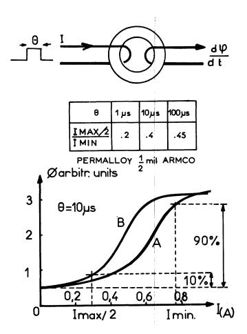
Figure 1—S-curves 1/2 mil thick etched permalloy toroids
