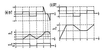
Figure 7—Composition of CRT deflection and beam waveforms
