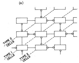
Figure 9a—Alternating type 1/type 2 cells in the multiplier matrix
