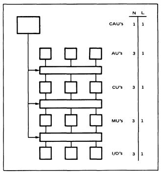
Figure 2—Three column modular computer
