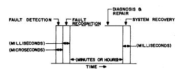
Figure 1—Fault recovery sequence (without spare)
