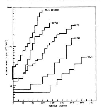
b. Pinhole density for silane-vapor-plated and R-F sputtered Si0<sub>2</sub> on delineated aluminum 5,000 Å and 10,000 Å thick
