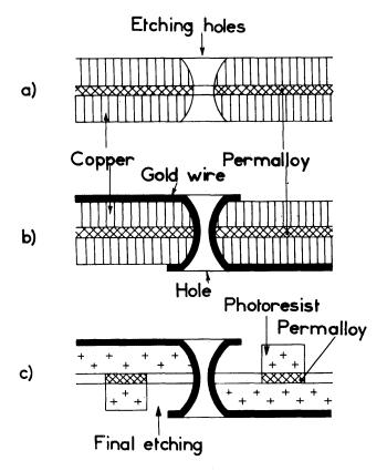
Figure 4—The new fabrication process: cross sectional view
