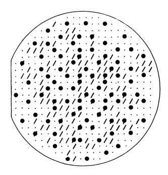
Figure 4—Master pattern superimposed on the particular yield of the Figure 2 wafer
