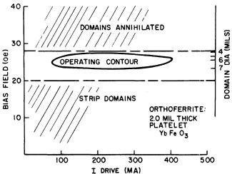
Figure 7—Quasi-static operating contour for 2-0 mil thick platelet of YbFe0<sub>3</sub>.
