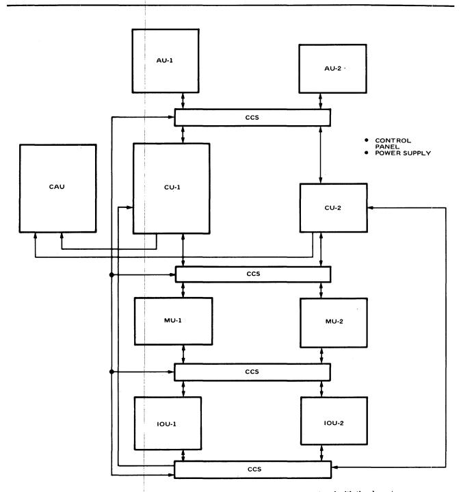
Figure 5—Block diagram of existing modular computer breadboard overlayed with the character implementation shown in Figure 6.
