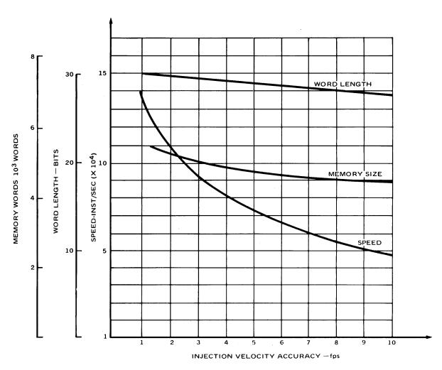
Figure 2 - Computational requirements for injection into parking orbit
