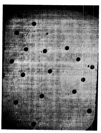
Figure 2—With a 42 Oe bias field the single wall strip domains of Figure 1 become cylinders each 1.8 mils in diameter
