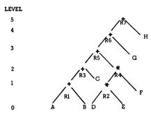
Figure 11—Parallel computation of A+B+C+D\*E\*F+G+H using Hellerman's algorithm
