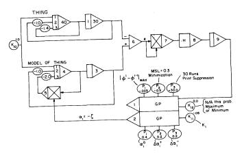
Figure 2-MOBSSL block diagram for second-order system damping ratio example
