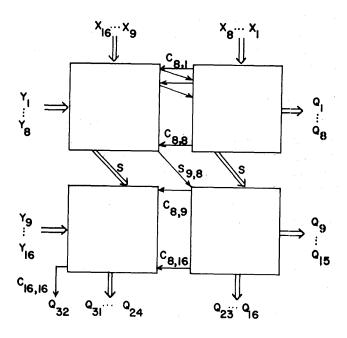
Figure 7—16  $\times$  16 bit functional multiplier on four LSI dies
