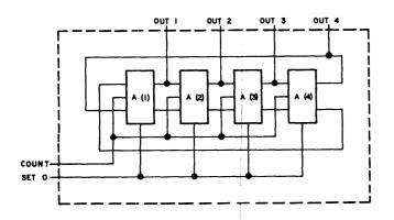
Figure 2—Four bit ring-counter
