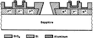
Figure 6—Final device structure
