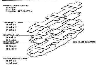
Figure 1—Storage element (exploded view)
