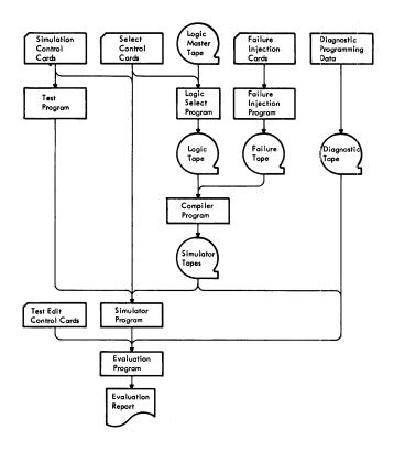
Figure 1—Simulator flow diagram
