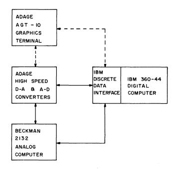
Figure 10—USC system simulation laboratory computer complement
