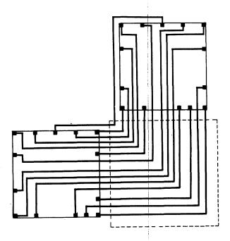
Figure 6—A set of pad relocations necessary to replace functionally the quad two-input gate circuit in area A of Figure 5
