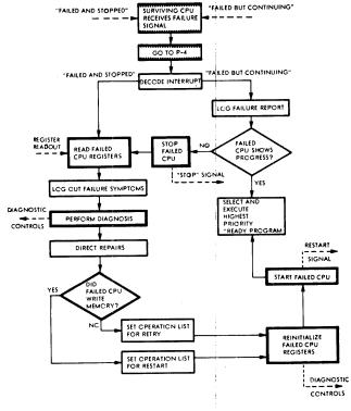
Figure 7— Central processor error: Surviving CPU
