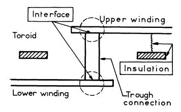
Figure 3—Cross sectional view of an ordinary integrated toroid
